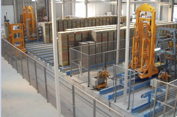
Sliding-bed machine RSM + flat stacking system RFS + transfer car system RAS + packaging
