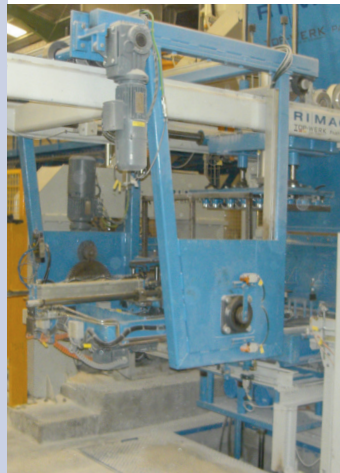
Sliding-bed machine RSM + turner RW 180° + matrix return RMR + racking system mobile RAC
